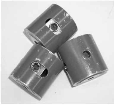
Figure 3. Each vertex has three holes: one circular, one hexagonal and one square. Only the configuration of figure 4 is allowed.
